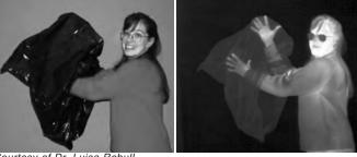
easily travel through glass. Since this person's body heat cannot travel through her glasses, they appear dark. Because infrared light can pass through dust, astronomers use infrared telescopes to study objects in space, like newly forming stars, which are hidden behind thick clouds of dust and gas. These new stars cannot be seen by visible light telescopes.
