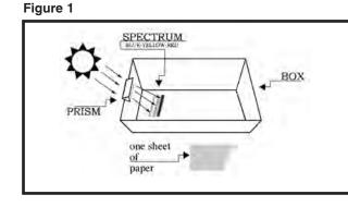
**MATERIALS:** One glass prism (plastic prisms do not work well for this experiment), three alcohol thermometers, black paint or a permanent black marker, scissors or a prism stand, cardboard box (a photocopier paper box works fine), one blank sheet of white paper.
