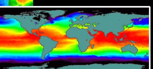
Infrared images allow us to remotely map cloud temperatures, even over oceans and at night. These measurements provide invaluable information about cloud heights and the destructive strength of hurricanes.
