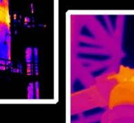
Power companies use infrared cameras to detect overheating or faulty connections in transformers and substations, allowing them to be fixed before they might cause a power-outage.
